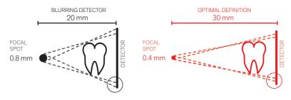
Increased X-ray parallelism and an incorporated collimator allow the RXDC to achieve a source-to-skin gap of 30 cm. The RXDC provides pin-sharp, precise images with outstanding detail.
